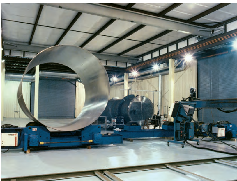
20,000 sq. ft. climate controlled clean room for titanium and zirconium fabrication.
